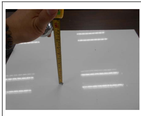
Finish impact test
