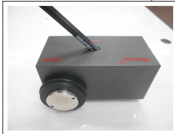
Paint Hardness on Steel Test Set-up
