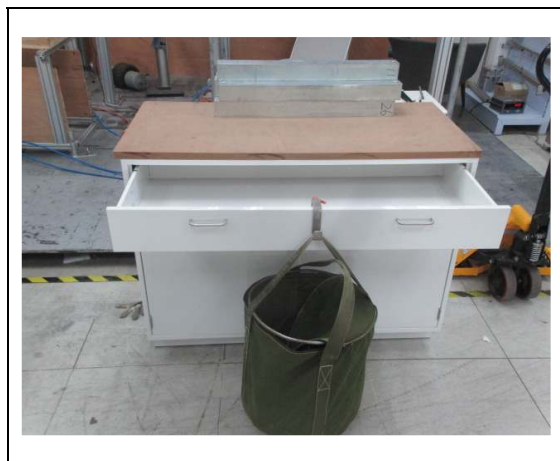
Drawer Static Load Test
